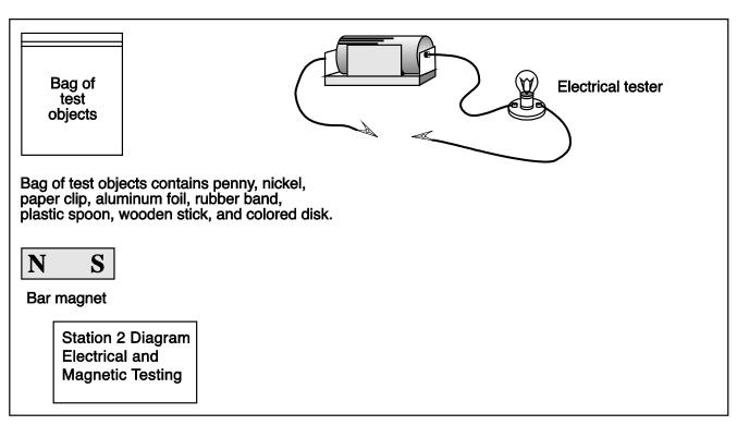
Station Diagram Station 2 — Electrical and Magnetic Testing
